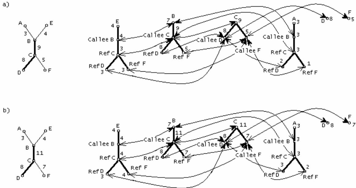
**Figure 4. CC-Map for Fig. 2 examples. Bold arrows indicate references from nodes describing call in a given context, thin arrows indicate references from a general information node to call-in-context nodes (this association is represented by “Context” items on Fig. 3). The roots of the trees are MethodProfile nodes containing the total counters for method executions**
