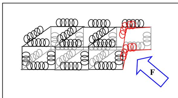
**Figure 2 Mechanical springs network with deforming force**
