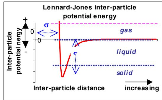
**Figure 1** Lennard-Jones potential modeling attraction or repulsion between two particles of an arbitrary material
